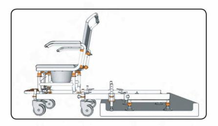
With the wheeled base, bridge and shower base securely connected together using the latches check that the entire length of the track is level horizontally.
