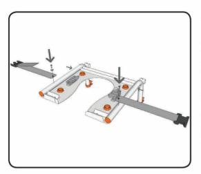
On the underside of the seat base there are 4 attachment points for the lap belt.
