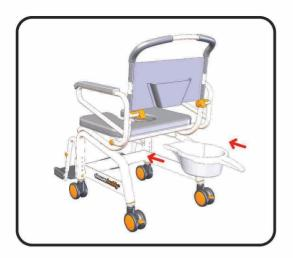
The Commode Bucket (part #500-072) can be pushed into position from the rear of the chair and is held in position by the Commode Bucket rails (part #500-362) pre-fitted to the cushion at the factory.
