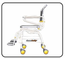
The chair may be adjusted to have a higher seat height at the front and lower at the back to suit user requirements. This can be accommodated by adjusting the front caster leg only to be extended further than the rear caster leg. Under no circumstances should there be more than 1-adjustment position difference between front and rear (approximately 20mm).
