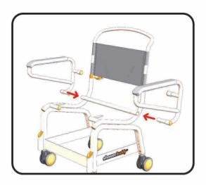
Fit Left Hand Arm (part #500-367) and Right Hand Arm (part #500-369) by positioning the axle (smaller diameter) part of the tube against the hollow tube across the rear of the Seat Frame (part #500-373/378) and sliding into this tube.
