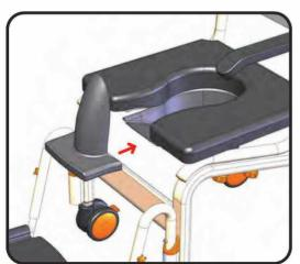
A Commode Deflector (part #500-074) is able to be fitted to the Commode Bucket after the bucket is fitted to the chair. The deflector may be fitted after the User is seated to allow easier transfers of the User to and from the chair
