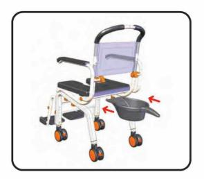
The Commode Bucket (part #500-072) can be pushed into position from the rear of the chair and is held in position by the Commode Bucket Connectors (part #500-095) pre-fitted to the cushion at the factory.
