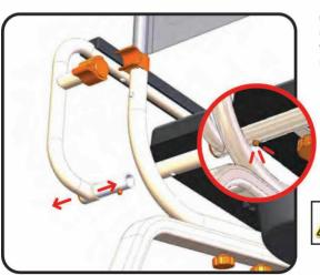
depress the push pin (part #500-269) fully allowing the arm rest to be pulled outwards from the seat frame tube. To re-fit the arm, reverse this action.
