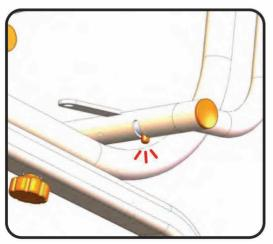
Once fully inserted the Push Pin will "pop out" into the formed slot to lock the arm into position. This prevents the arm from being removed again without depressing the Push Pin.
