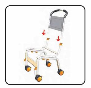
Slide Back Rest Frame (part #500-042) down through Arm Clips (part #500-237) and into the Seat Frame (part #500-021). Make sure that push pins are fully depressed before inserting the back rest frame.
