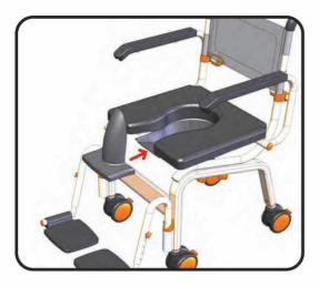
A Commode Deflector (part #500-074) can be fitted to the front of the commode bucket if required, after the bucket has been fitted to the chair, allowing the user to transfer easily to the chair prior to fitting the splash guard.
