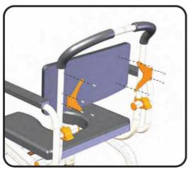
To install, simply remove the safety restraint clamp bars (part #500-106) and replace them with the two back rest support arms shown.
