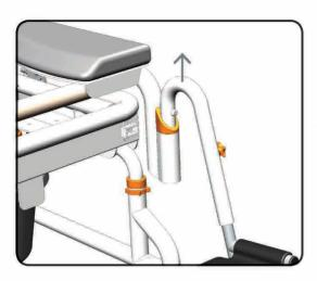
To swing the footrest out of the way simply lift the leg out of the slot and spin the leg away.
